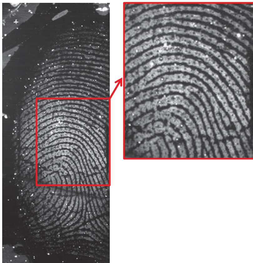
Figure 4-18 One-week-old natural fingerprint half deposited by a male donor on aluminium foil, developed with the working solution containing Sequence #5, and visualised at 530 nm with a 590 nm bandpass filter.
