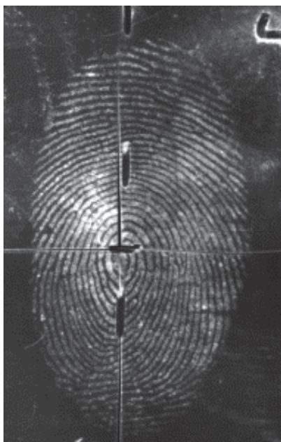
Figure 2-11 Natural fingerprint deposited on PVDF and processed for 15 minutes (top right), 30 minutes (bottom right), 45 minutes (top left), and one hour (bottom left), visualised at 590 nm with a 650 nm bandpass filter.
