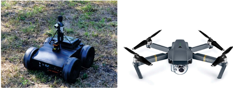
FIGURE 1.1: Examples of robots that need solutions of SLAM and VINS: the automated guided vehicle and the unmanned aerial vehicle
