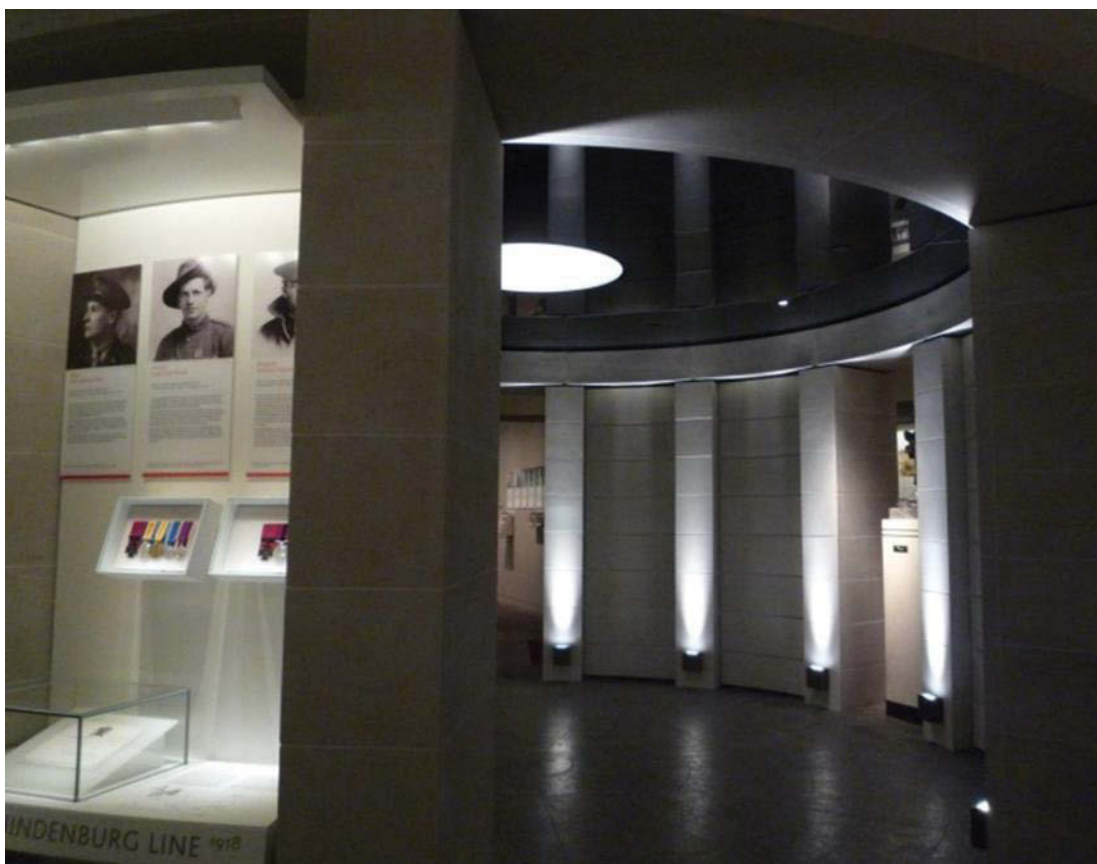
Figure 1.8: Australian War Memorial, Canberra utilises Light-emitting Diodes for the lighting of display niches (Photo: Mirjam Roos, Steensen Varming, 2011)
