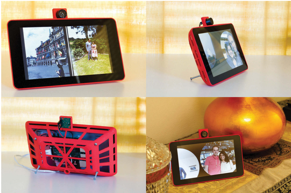
Figure 8.1. The Phototype device, showing (in clockwise order) the DualDisplay mode, the PhotoSoup mode, its back, and placed on a dresser table.
