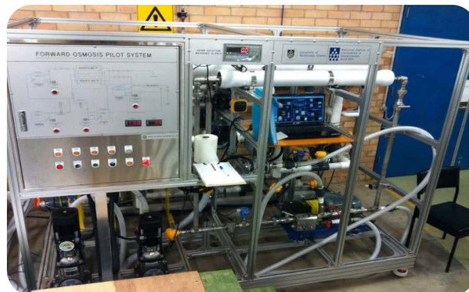
Figure 3 - 5. A schematic diagram of (a) FO process, (b) NF process and (c) a photo of pilot-scale FDFO-NF hybrid system installed at University of Technology Sydney (UTS)
