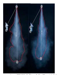
Fig. 2 (a) Spray angle of B100 (left) and distillate (right) at 0.4MPa. (b) Spray tip penetration of B100 (left) and distillate (right) at 0.4MPa.
