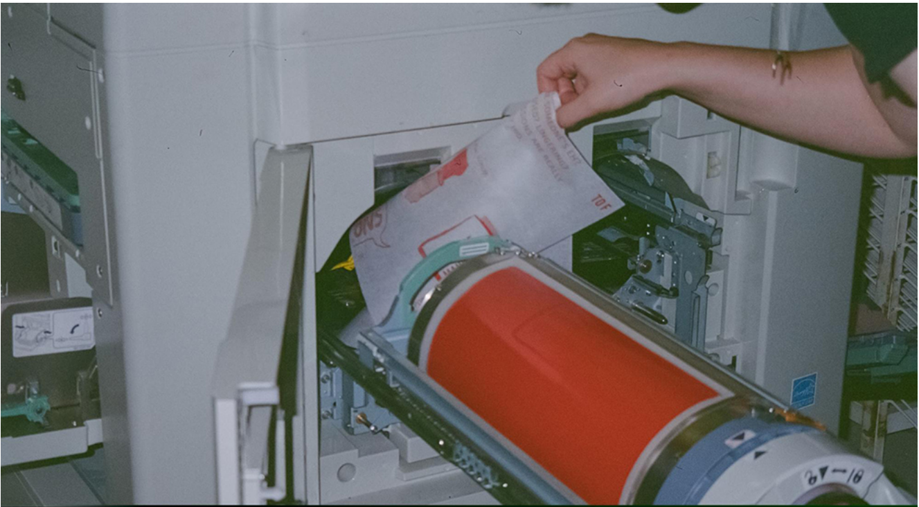
Figure 4: Pulling the translation off the drum; this was done every print making the process slow and requiring gentleness.
