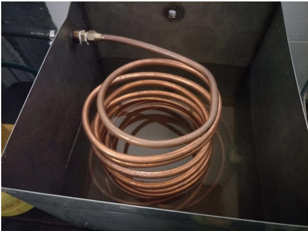
Figure 54 Condenser Coil (Coil OD: 200 mm)
