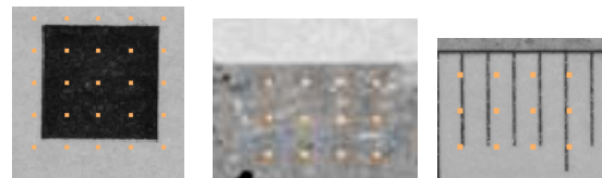
Figure 7. Three types of specimen surface: printed pattern, concrete surface and scale mark
