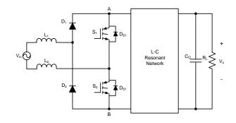
Figure 5: A TPBBR topology with L-C resonant network.
