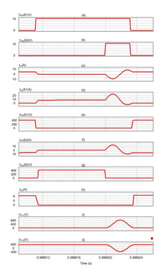
Figure 9. The SPBBR simulation results at 240 Vin<sub>rms</sub> (a) Gate signal for S1. (b) Gate signal for S2. (c)  $i_{Lr}$ . (d) Current through S1. (e) Voltage across S1. (f) Current through S2. (g) Voltage across S2. (h) Current through diode D3. (i) Voltage across resonant capacitor  $C_{r1}$ /diode D3 and (j) Voltage across resonant capacitor  $C_{r2}$ .
