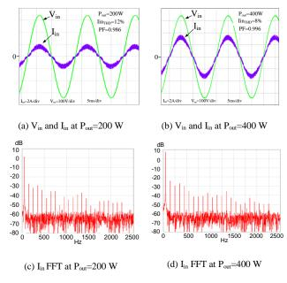
Figure 10. Simulation results of input supply voltage, input supply current, and corresponding FFT for SPBBR at different loads
