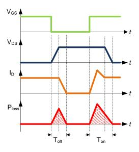
Figure 3: Losses in between switching transition.
