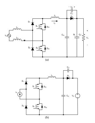
Figure 6: (a) Proposed SPBBR converter topology (b) Equivalent circuit of the proposed SPBBR converter topology during steady-state.
