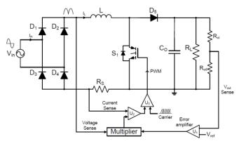
Figure 1: Typical circuit of CCM boost PFC rectifier
