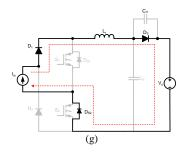
Figure 8: Equivalent circuit of the proposed TPBLB converter during positive half cycle (a) Interval 1 (b) Interval 2 (c) Interval 3 (d) Interval 4 (e) Interval 5 (f) Interval 6 (g) Interval 7.
