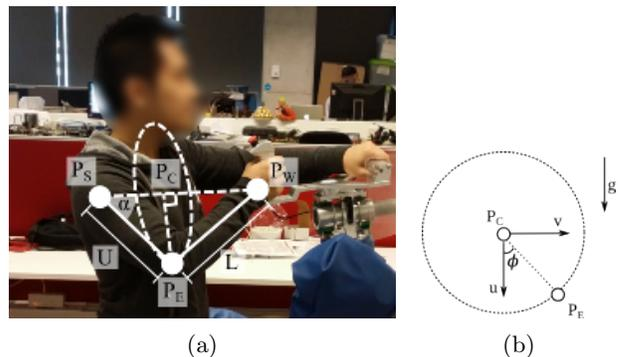
Figure 2: a) Location of the swivel coordinate frame  $P_C$  in relation to the subject’s shoulder  $P_S$ , elbow  $P_E$  and wrist  $P_W$  b) Swivel coordinate frame  $\vec{u} \times \vec{v}$  showing the swivel angle  $\phi$  and direction of gravity  $\vec{g}$ .
