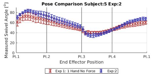
Figure 7: Comparison of the mean swivel angles for Experiment 2 and Experiment 1
