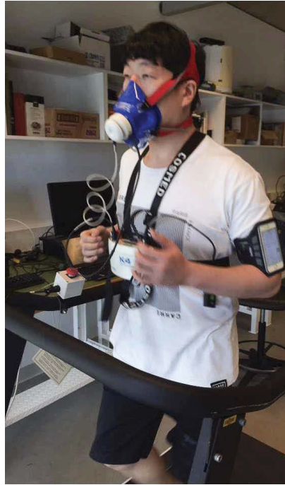
Fig. 6.8 The LabVIEW controlled treadmill system for experiments
