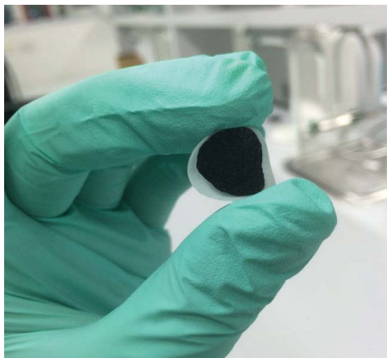
Figure 6-6. Digital photograph of the \text{Na}_3\text{V}_2(\text{PO}_4)_3@\text{CP} hybrid electrode slightly bent to demonstrate its structural integrity under stress.
