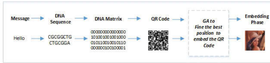
Fig. 24.1 Flowchart of the Proposed Method of DNA with QR Code
