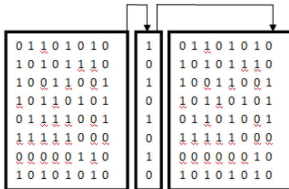
Figure 2.16.: LSB coding method (Kaur, 2015)
