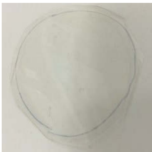
Figure 29: Nafion-117 Cut to either 25 or 40 mm Diameter for use as a Membrane in the DCMFC
