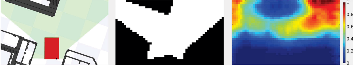
FIGURE 4.6: CNN generation of a traversal heatmap (right) from the occupancy map (centre) corresponding to the LIDAR readings (green) in the left image.
