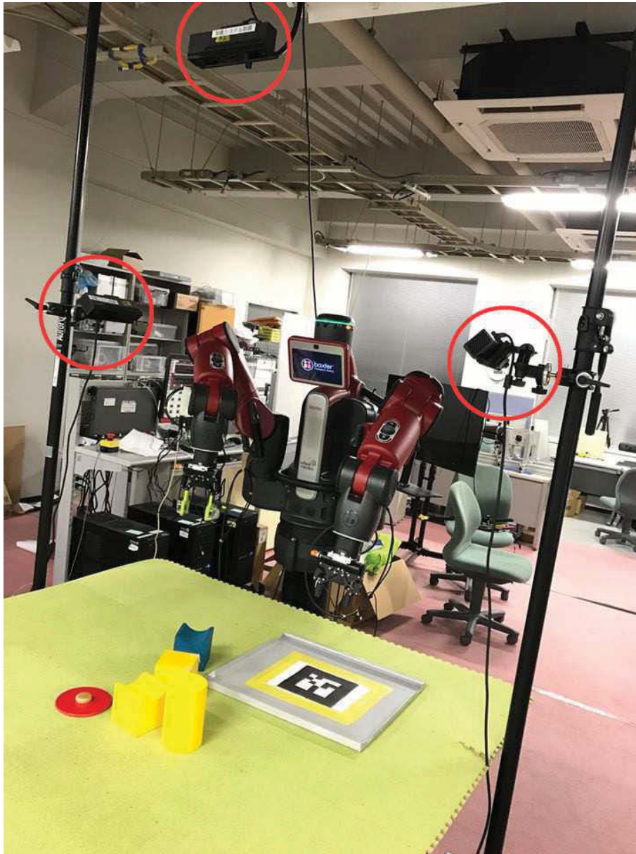
FIGURE B.1: Complete Baxter setup at NAIST during extrinsic Kinect calibration. The black-and-white pattern on the table is the AR marker. Kinect units are circled in red.
