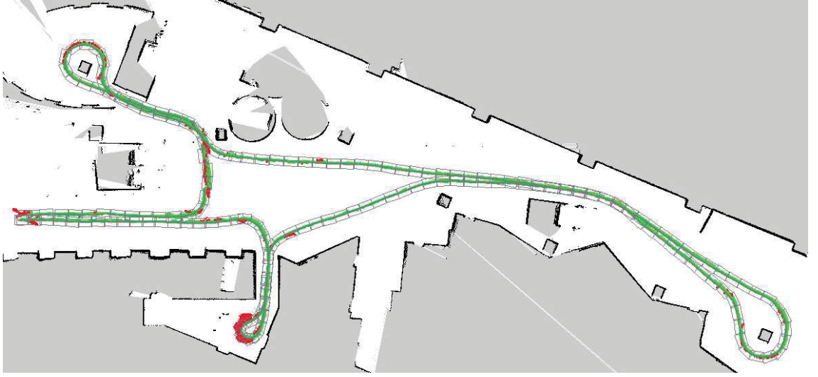
FIGURE 3.16: Visualization of the intention estimator and path generator, run a-posteriori for each of the logged points along an able user's free path. More details available in Section 3.5. Conducted on UTS campus in a space measuring approx. 60 \times 27m , on the CAS wheelchair.
