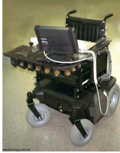
FIGURE 2.1: The Navchair intelligent wheelchair with on-board PC and ultrasonic sensor array, capable of obstacle avoidance and pre-programmed behaviors such as wall following and doorway navigation.
