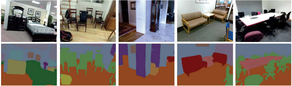
FIGURE 4.2: Example segmentation of image scenes via CNN semantic mapping. From Badrinarayanan et al. (2015).
