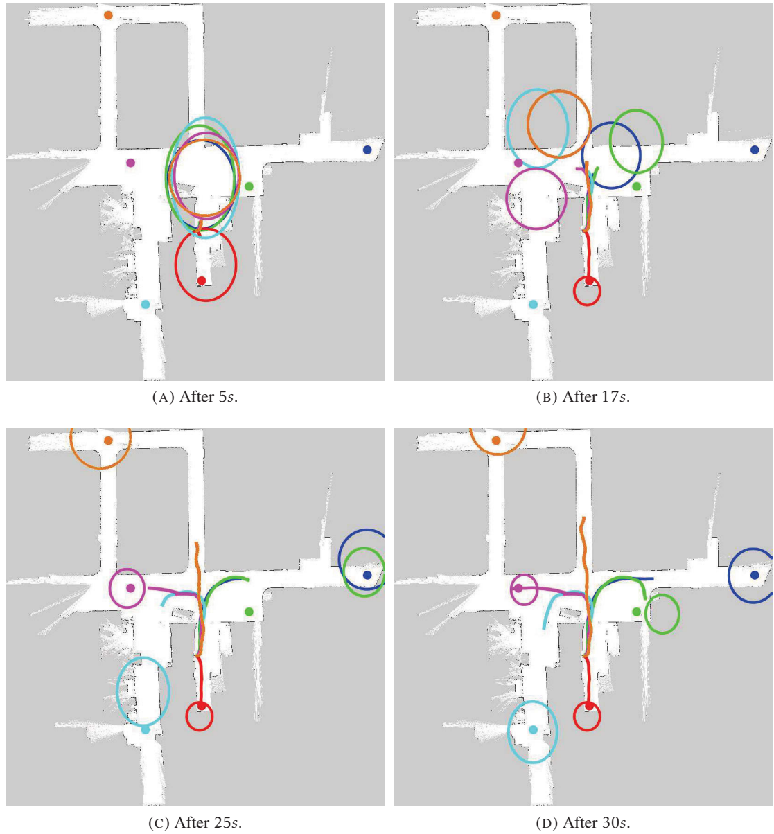
FIGURE 2.6: Illustrative examples of user intention estimation with the full GP user action model. The six goals are indicated by points of different colours, with their corresponding trajectories and GP ellipses in matching colour. By 30s, all the ellipses have almost reached their goals with reduced covariances.
