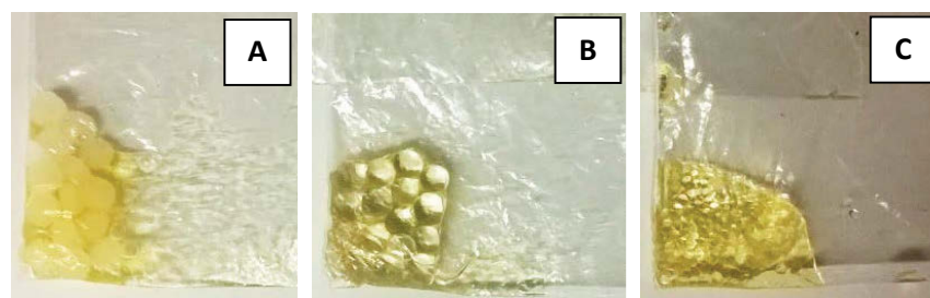
Figure 4-4. Test results using a combination of PE bag and microbeads performed with addition of 4-MMC after 5 min using A) PE pellets (Exp 3-1), B) glass beads (Exp 3-2) and C) PVAc solid resins (Exp 3-3)
