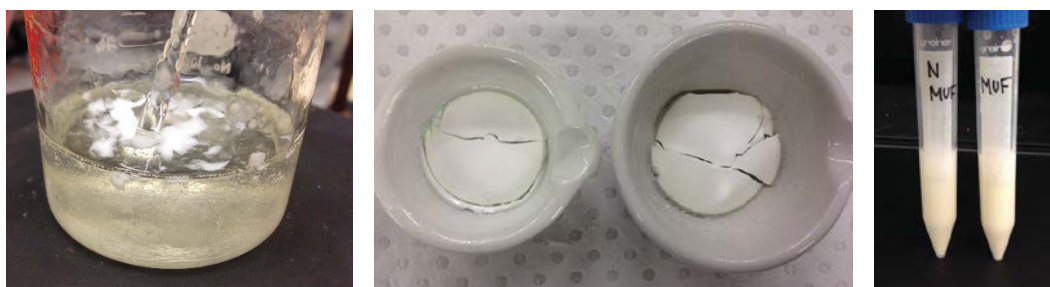
Figure 6-6. Preparation of MUF resins for selective adsorption: A) MUF gel mixture prior to incubation, B) imprinted and non-imprinted MUF resins after incubation, C) grinding MUF resins in mortar and pestle
