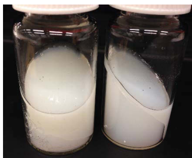
Figure 6-3. The polymerised solutions of ephedrine imprinted (left) and non-imprinted (right) polymers (pol-3)
