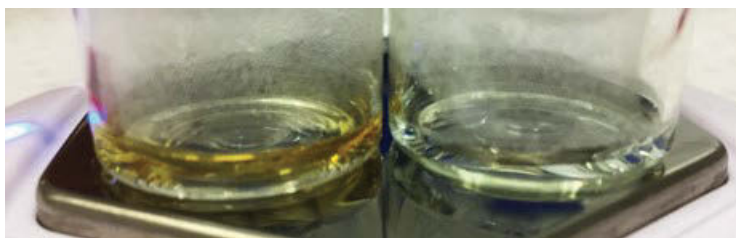
Figure 4-5. Result of colour test (Exp 4-1) performed on 4-MMC as a positive control ( left ) and control reagent blank ( right ) using USB-powered mug warmer after 10 minutes of heating
