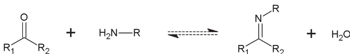
Figure 1-9. Reaction equation for the formation of an imine from a ketone
