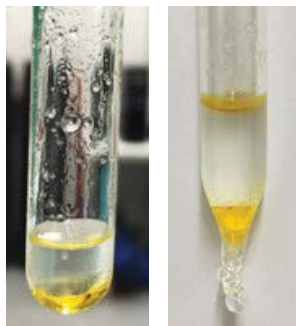
Figure 4-11. Colour test result employing chloroform as an organic extraction solvent to concentrate the coloured product performed in A) a semi-micro test tube and B) a sealed Pasteur pipette
