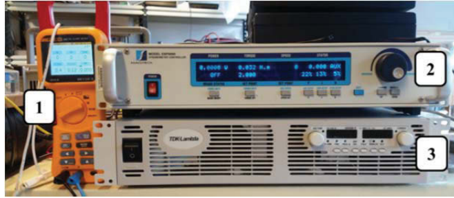
Fig. 5.4.2 Platform setup of experimental test, where (1) power quality clamp meter, (2) dynamometer controller, and (3) DC power supply.
