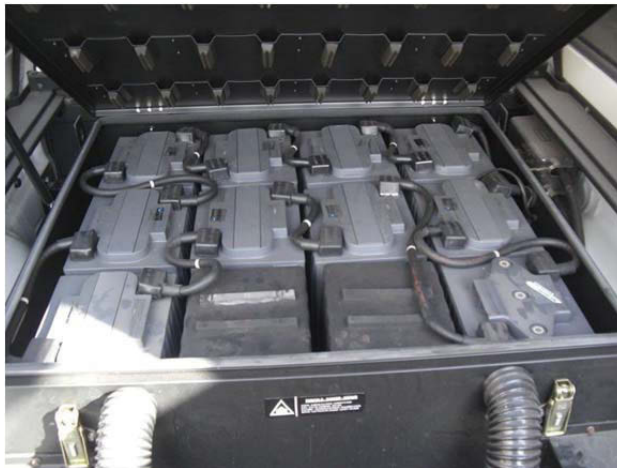
Fig. 2.4.5 The battery pack of Fiat Panda Elettra (from [2.51])
