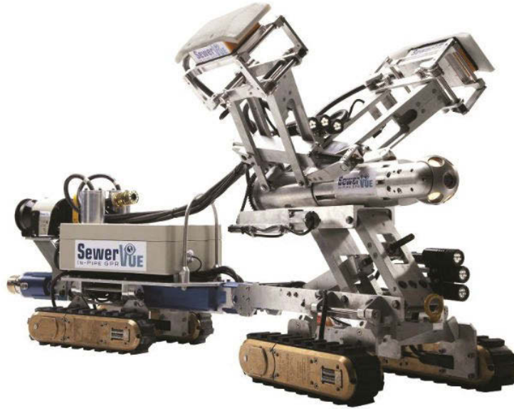
FIGURE 1.1: Multi-sensor robot for condition assessment of sewer infrastructures [1].
