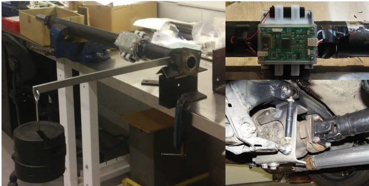
Figure 9-21: B-DAQ Torque Sensor Calibration.
