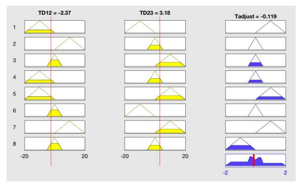
Figure 9. Visual process of input [-2.37, 3.18] in FLS for output T<sub>adjust</sub>.
