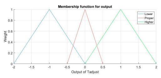
Figure 8. Membership functions for output T<sub>adjust</sub>.
