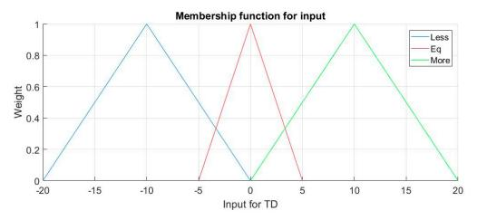
**Figure 6.** Membership functions  $\mu(x)$  for input TD<sub>12</sub> and TD<sub>23</sub>. TD: temperature difference.
