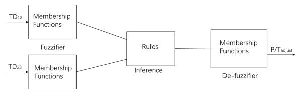
Figure 5. Data structure of fuzzy logic system for  $P/T_{adjust}$ .
