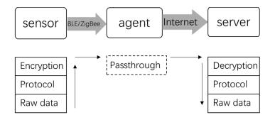
Figure 1. Data-flow block diagram of system.
