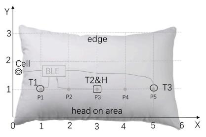
Figure 4. Physical structure of smart pillow as Cartesian coordinates.
