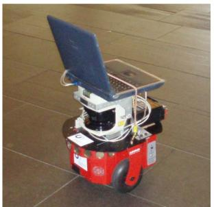
Figure 4: Pioneer 2DX used for LAM and PPOA development.
