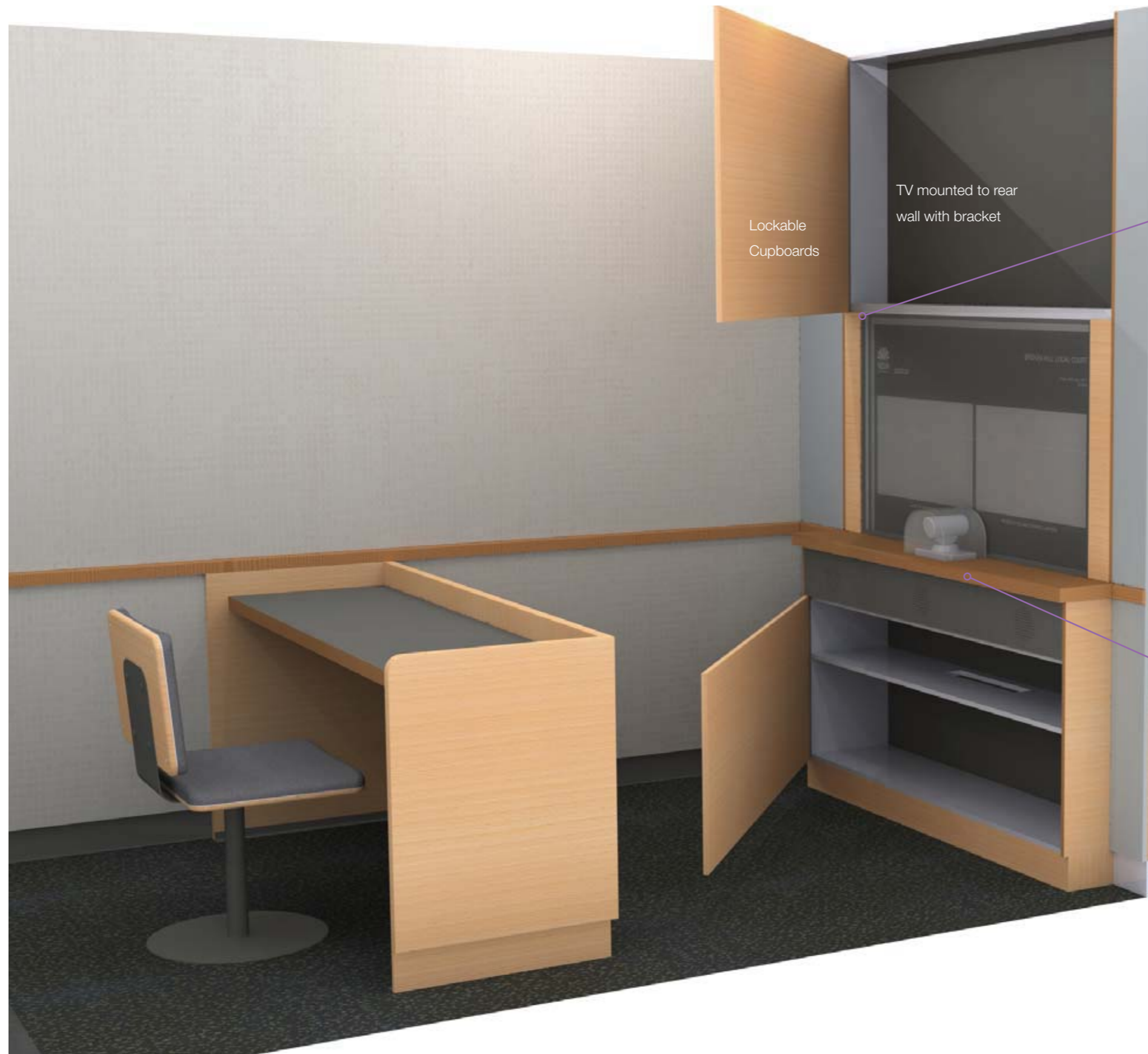
Lexan slides into steel C sections. Can be removed by opening top cupboard
