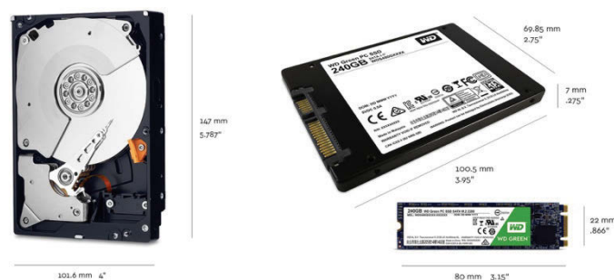
Figure 2.8: Internal hard drives. Western Digital WD Black (left); Western Digital WD Green PC SSD (right) (source: www.wdc.com )
