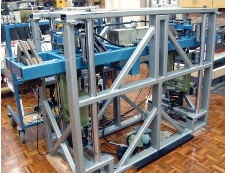
Figure 3.1: Half-Car Testing Rig designed and built by Wade Smith and Chris Chapman in 2005
