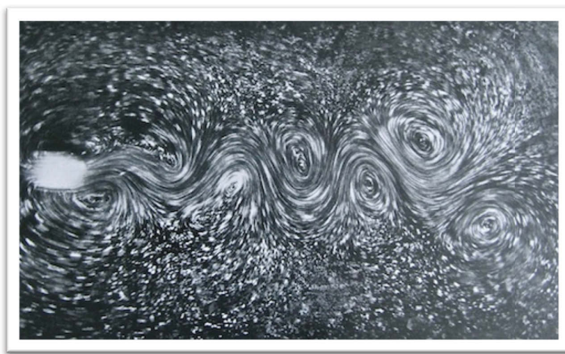
Figure 6.1: Meander and vortices in water flow
