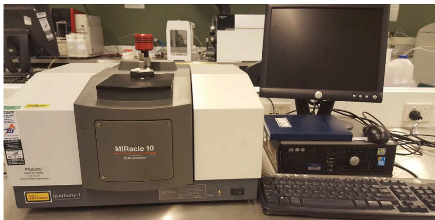
Figure 3 - 10. Attenuated total reflectance-Fourier transform infrared spectroscopy (ATR-FTIR) equipped with a single reflection ATR accessory.
