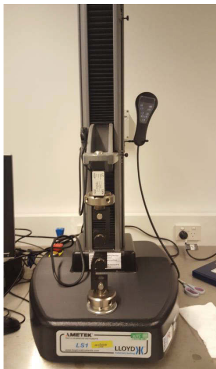
Figure 3 - 11. Advanced Testing System (LS1, Lloyd instruments Ltd, UK) for evaluating mechanical properties of membranes.
