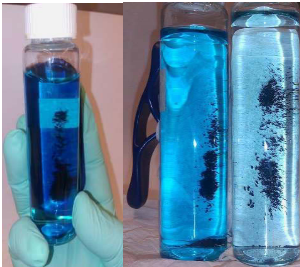
Figure 4.4.18: Use of a magnet bar to demonstrate easy separation of n\text{Fe}_3\text{O}_4\text{-fBC} composite after experiments.
