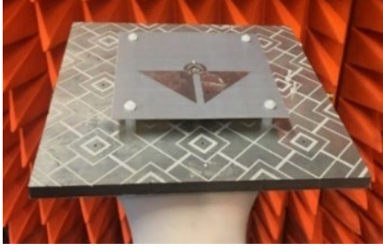
Fig. 5. Fabricated prototype of the wideband CP reconfigurable antenna with the AMC ground.
