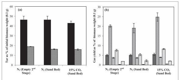
**Figure 2.** (a) Tar yields and (b) detectable gas yields produced from the fast pyrolysis of 0.100 g of beech wood in different gaseous environments in the single-stage (filled bars) and two-stage reactor at 973 K (pattern filled bars) with and without a sand bed in the 2nd reactor stage. Tar (black bars), CO (dark grey bars), CO<sub>2</sub> (light grey bars) and  $CH_4$  (white/polka dot filled bars).
