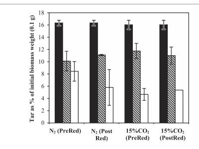
**Figure 3.** Comparison of the tar yields produced after exposure to the sand beds at 973 K under the different inlet gas compositions (filled bars) and simulated CLC experiments in which the 100Fe(S) OCM (pattern filled) and 60Fe40Al OCM (empty bars) was exposed to volatile pyrolysis products during the 3rd cycle reduction phase at 973 K.
