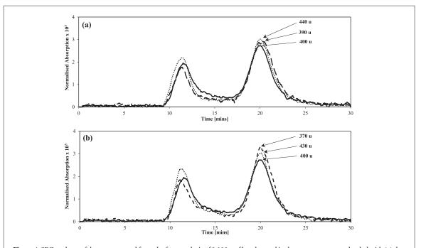
Figure 4. SEC analyses of the tar recovered from the fast pyrolysis of 0.100 g of beech wood in the two-stage reactor loaded with (a) the 100Fe OCM and (b) 60Fe40Al OCM in both their oxidised and reduced forms under a  $N_2$  atmosphere. Sand ( ——); 'PreRed' conditions (———); 'PostRed' conditions (———).
