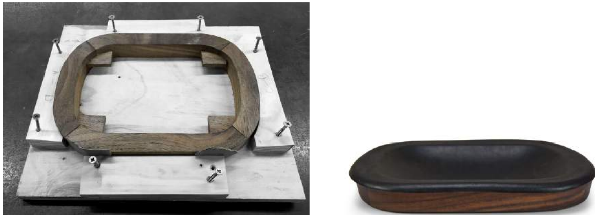
Figure 5: New Tray with Leather Lid made from 'Beanz' Tray tool. The 'timber loop' used to brace the original enamel tray is further machined and finely finished in American Walnut to act as a base in a new version of the design. The tool becomes the product ending the cycle for this series.
