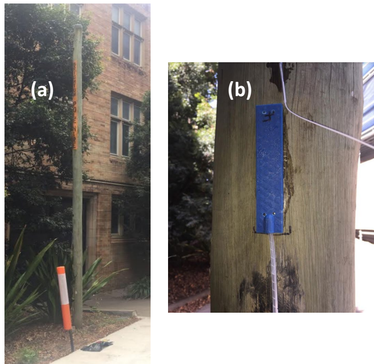
Figure 1. (a) An old, abandoned, timber, utility pole no longer in use at the University of Sydney; (b) A packaged FBG is placed approximately 1.3 of the way up the pole.
