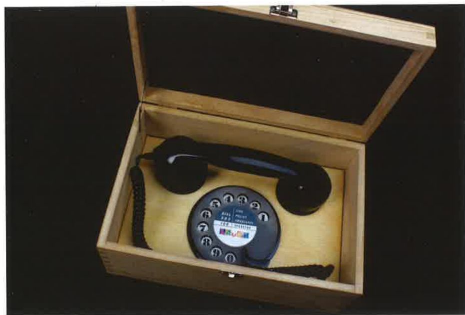
This telephone plays music and the sound of Spanish-speaking voices. It was designed for a woman who had grown up in Spain and loved hearing the Spanish language
