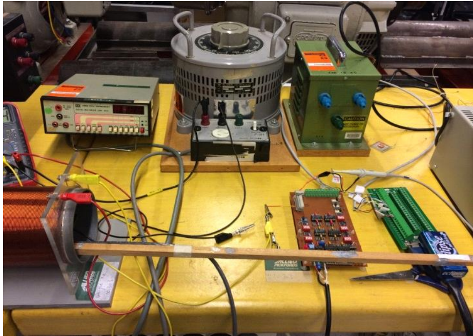
Fig. 3.3 Calibration of B and H sensing coils
