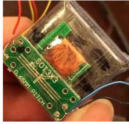
Fig. 3.1 SOMALLOY 700 (5P) cubic sample with sensing coils
