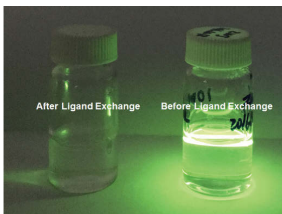
Figure 5-23. Comparison of visible emission between the cyclohexane layer before (a) and after (b) ligand exchange with CB[7] solution under 980 nm laser.
