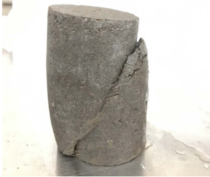
Figure 3.23 A selected sample after completion of triaxial shear test
