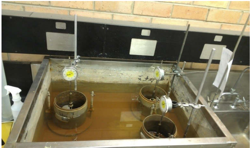
Figure 3.20 Swell potential test setup
