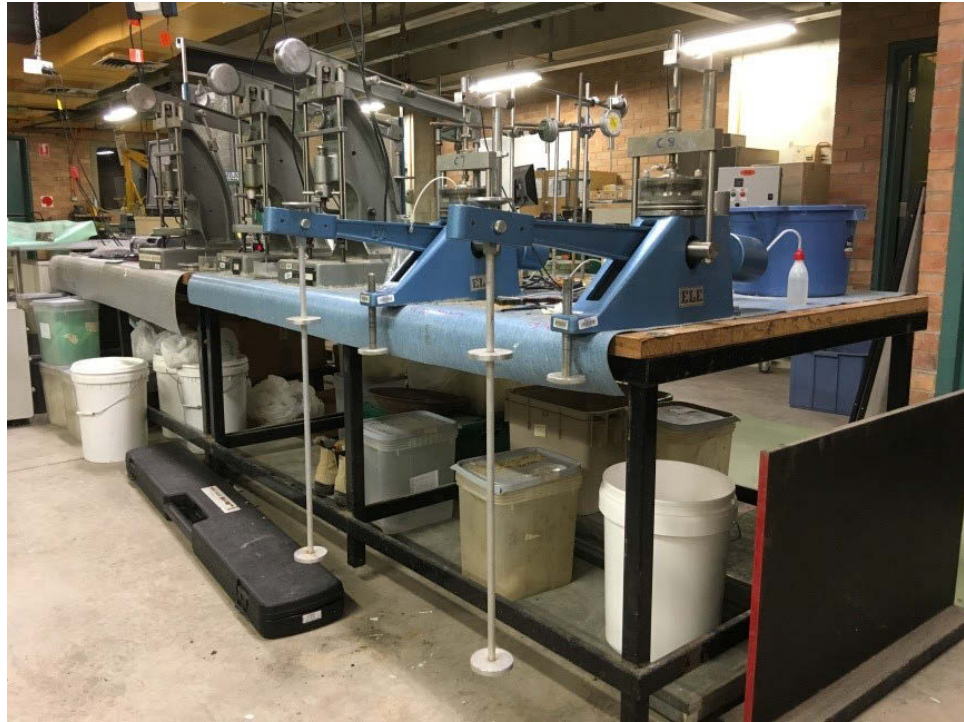
Figure 3.21 One-dimensional (1D) consolidation test (Oedometer test)
