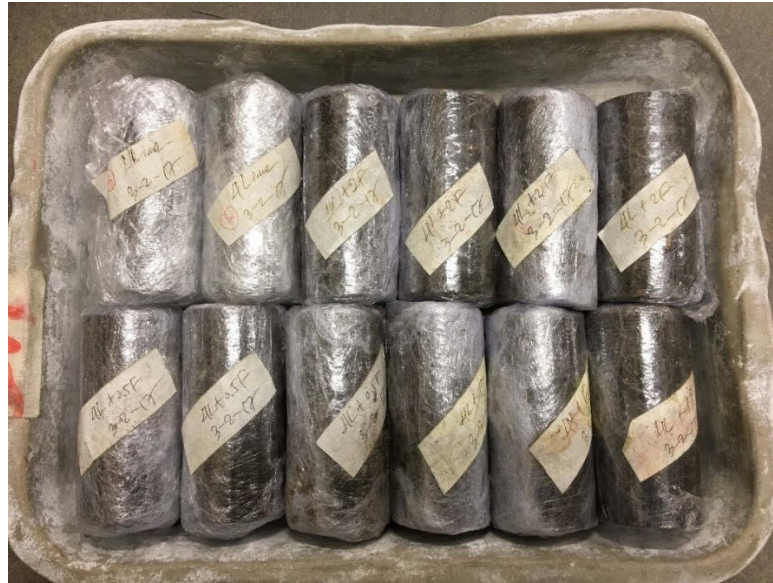
Figure 3.13 Unconfined compressive strength test: (a) a typical UCS mould; (b) selected soil samples prepared and sealed in vinyl plastic wrap for curing
