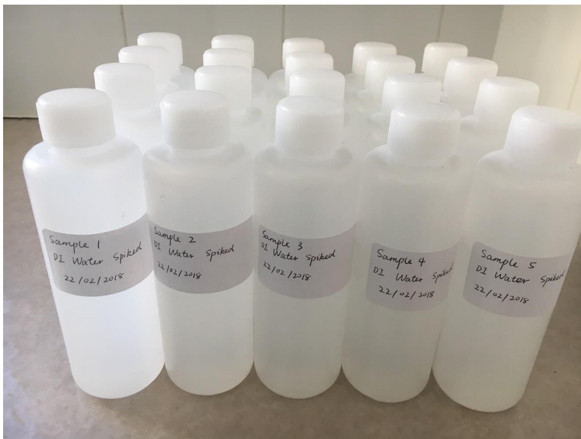
Figure 2. DI water samples (200 mL) were spiked with a multi-element standard solution.
