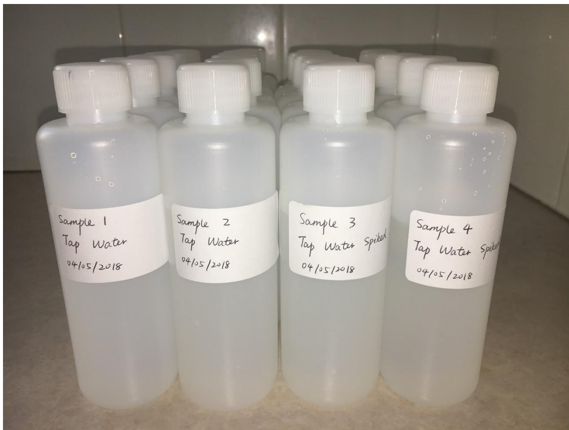
Figure 9. Drinking water samples (200 mL) spiked with a multi-element standard solution.
