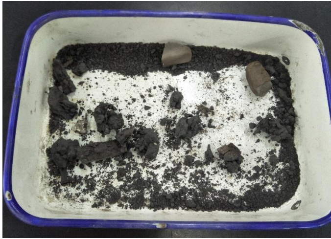
Figure 4.8. Debris of specimen suffering explosive spalling at 370 °C.
