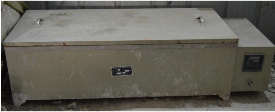
Figure A.3. Water tank with thermostatic control.
