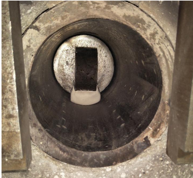
Figure 5.1. A specimen with a mat for dynamic splitting tensile tests.
