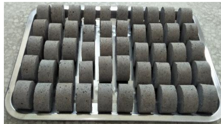
Figure 4.1. Specimens for SHPB tests.
