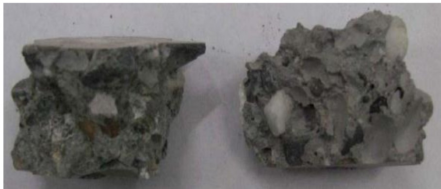
Figure 2.8. Damage characteristics under ambient (left) and 400°C (right) temperature (Jia 2011).
