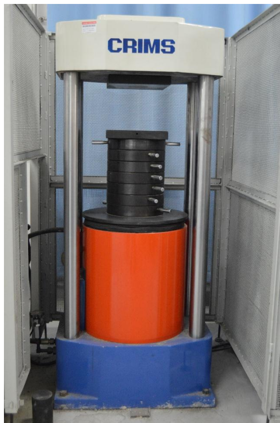
Figure A.2. 1000 kN capacity electrohydraulic servo pressure testing machine.
