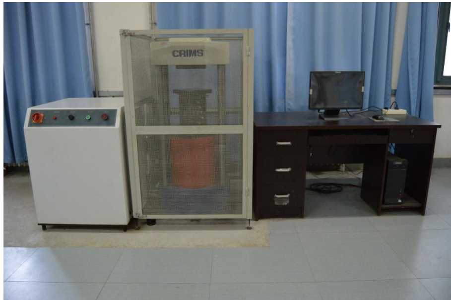
Figure A.1. Compression test setup.
