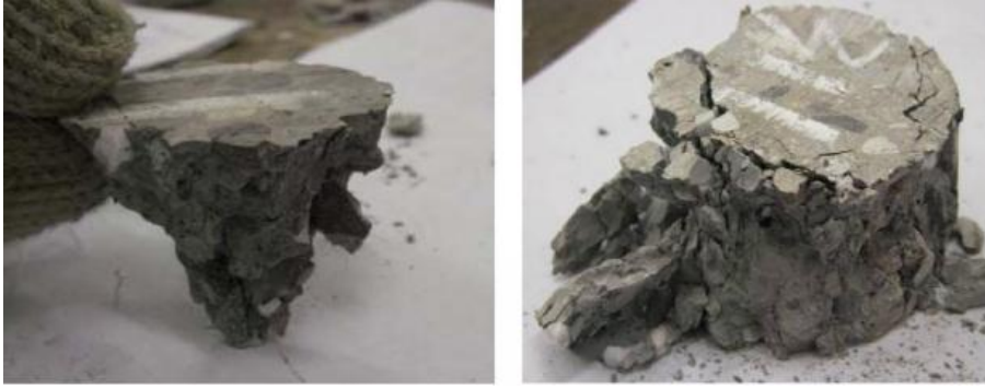
Figure 2.9. Two types of damage under 400°C (Jia 2011).
