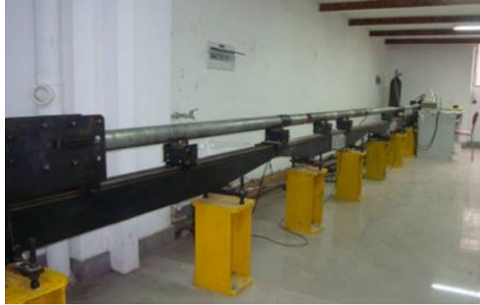
Figure 2.10 SHPB test setup (Huo et al. 2012).
