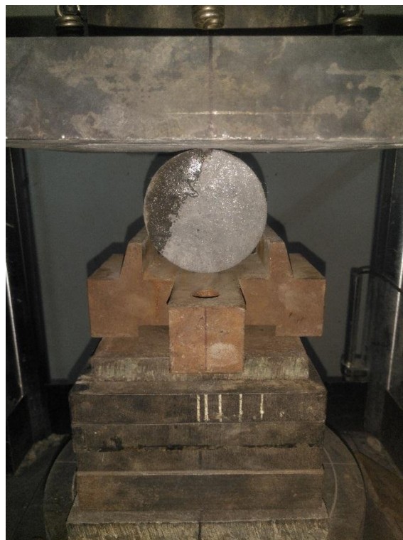
Figure 5.2. Setup of static splitting tensile tests.
