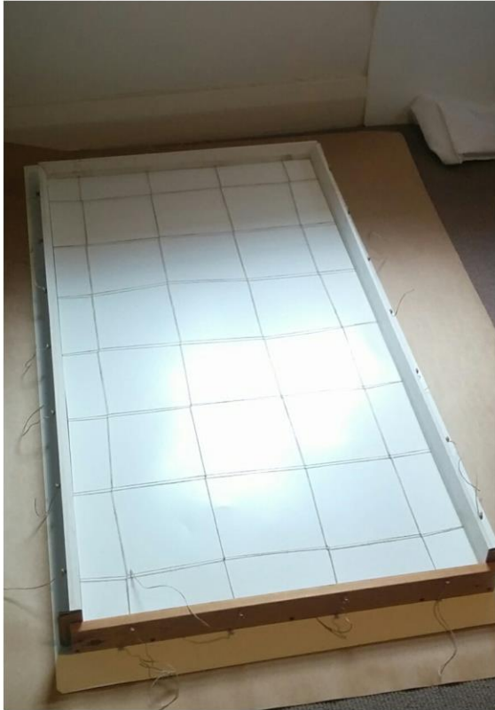
Figure 25: 1200mm x 650mm mould with twine reinforcements.
