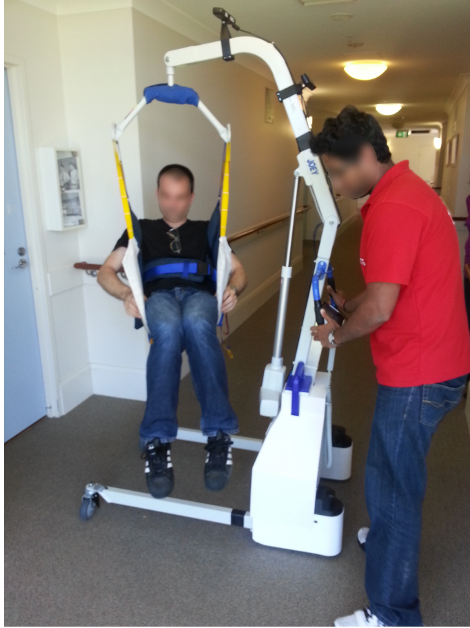
FIGURE 4.16: Smart Hoist: A robotic patient lifter designed to assist carers in transporting patients through pHRC.
