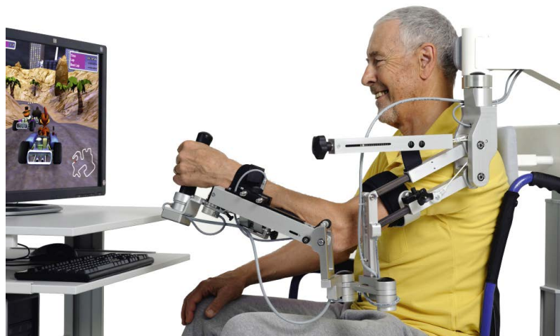
FIGURE 2.5: An example of an exoskeleton used for pHRC designed to assist in the recovery of stroke patients [9].
