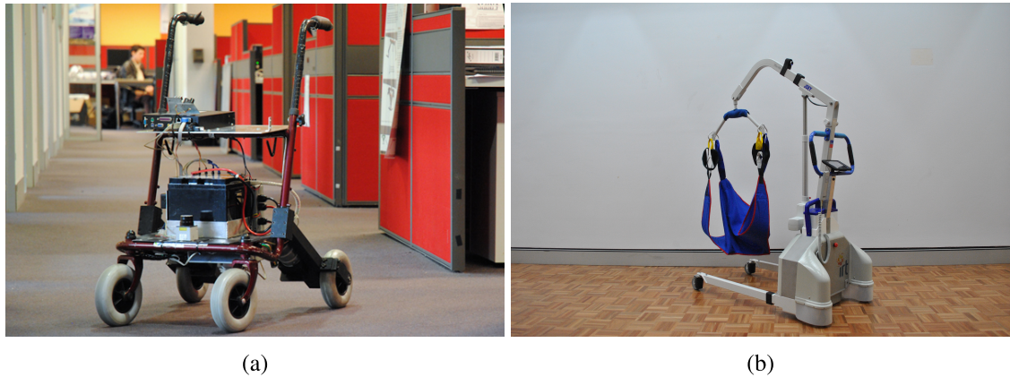
FIGURE 2.4: Examples of assistive devices which also have some of the technologies used in smart wheelchairs. (a) Smart walker [8]. (b) Smart Hoist.
