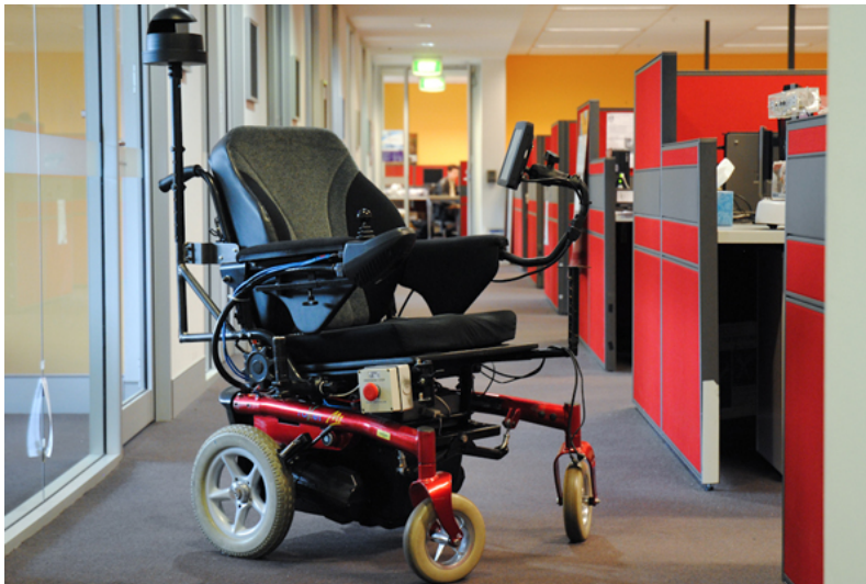
FIGURE 2.3: An example of a smart wheelchair used for pHRC capable of semi-autonomous navigation [8].
