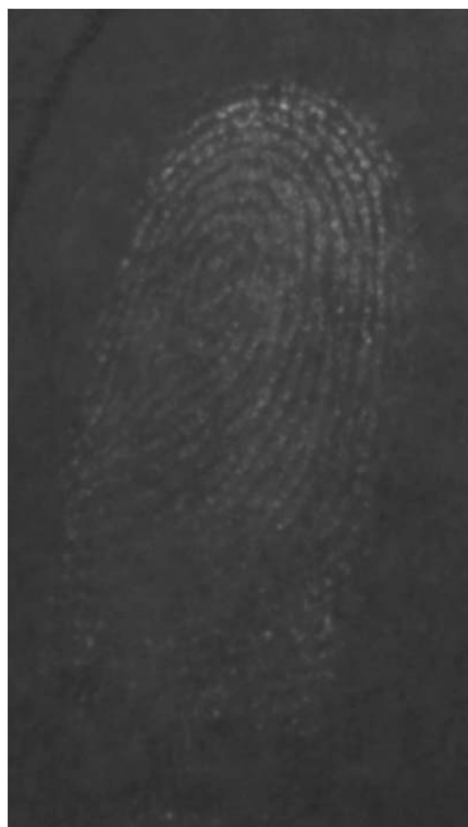
Figure 4-16 Ethanolic solution of zinc chloride 'washing' away some fingerprint ridges (bottom of the fingerprint).
