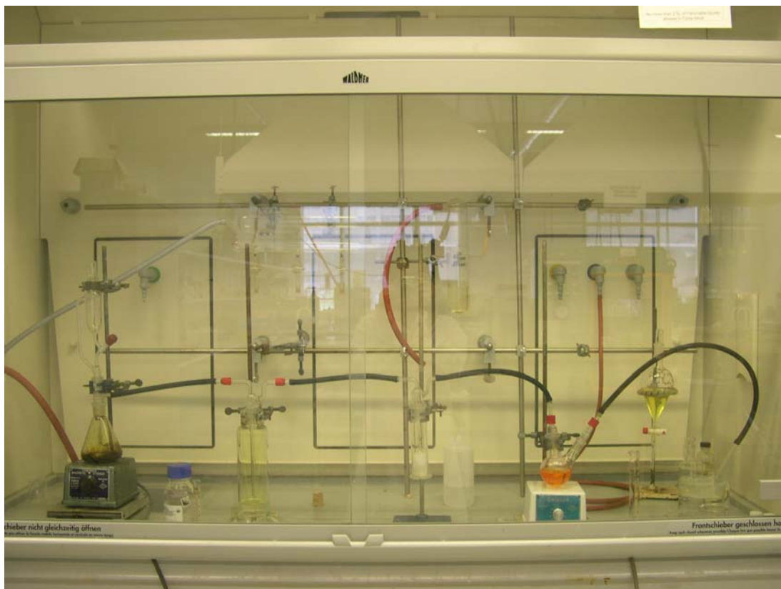
Figure 3-9 Reaction configuration in which chlorine gas is generated and bubbled into a solution containing 9-chloro-10-hydroxy-1,4-anthraquinone.
