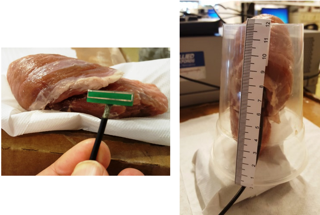
Figure 4-10. Measurement setup for Transmitter antenna on FR4.
