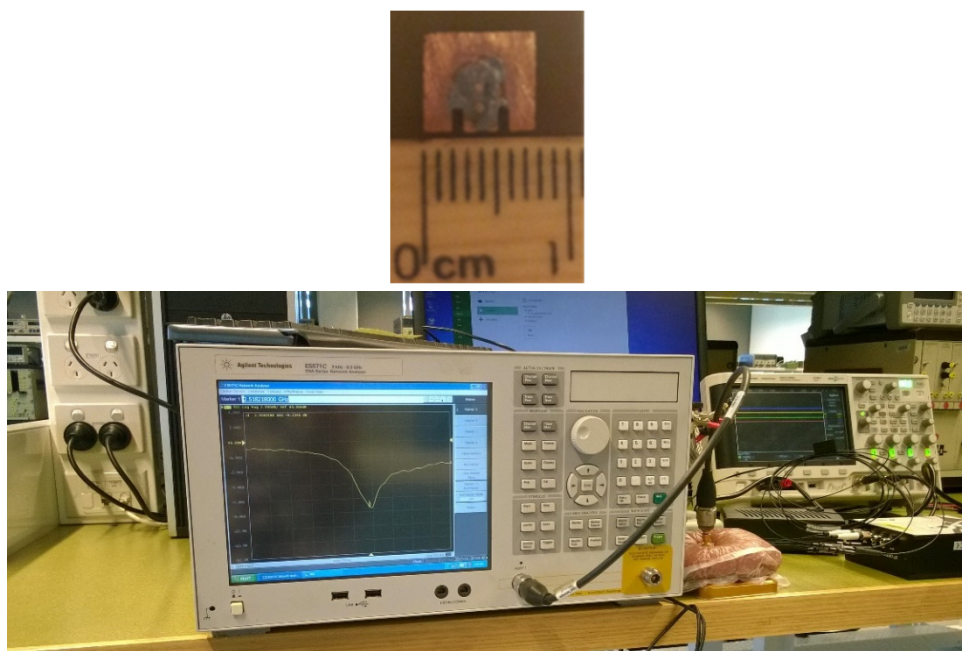
Figure 6-13. Printed Dual Slot PIFA on FR4 substrate and measurement setup.
