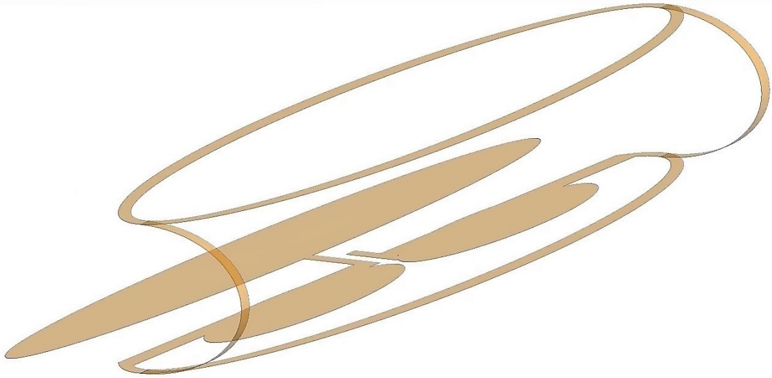
Figure 5-16. Wide band folded oval loop antenna geometry.
