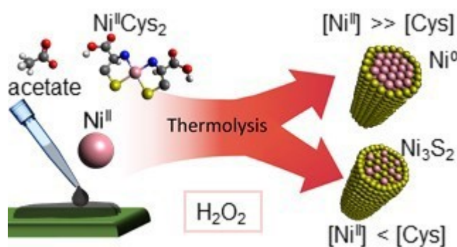
FIGURE 4.9: Schematic illustrating the precursors used in nanowire synthesis: \text{Ni}^{\text{II}} acetate and \text{Ni}^{\text{II}} bis-cysteinate, and the substrate preparation procedure. \text{H}_2\text{O}_2 was added to the \text{Ni}^{\text{II}} acetate and \text{Ni}^{\text{II}} bis-cysteinate precursor solution to achieve \text{Ni}_3\text{S}_2 nanowire growth. Following dropcasting and drying of the nickel-complex solution; nanowire growth of the \text{Ni}^0 and/or \text{Ni}_3\text{S}_2 phase is achieved by annealing in high vacuum.
