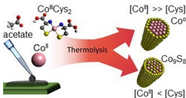
FIGURE 4.1: Schematic illustrating the precursors used in nanowire synthesis: \text{Co}^{\text{II}} acetate and \text{Co}^{\text{III}} bis-cysteinate, and the substrate preparation procedure. Following dropcasting and drying of the cobalt-complex solution; nanowire growth of the \text{Co}^0 and/or \text{Co}_9\text{S}_8 phase is achieved by annealing in high vacuum. Nanowire phase is determined by the \text{Co}^{\text{II}}:\text{Cys} mole ratio.
