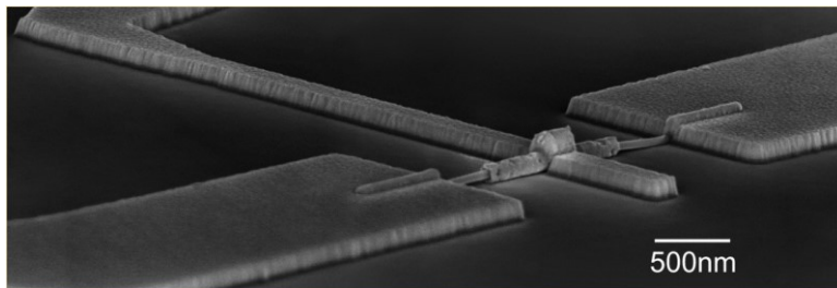
FIGURE 1.6: Wrap-gate nanowire field-effect transistor.[ 203 ]
