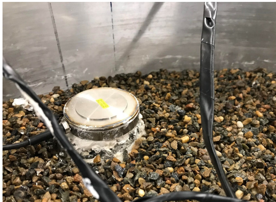
Figure A.6 Earth pressure cell (EPC) positioned and fixed on the CIC using plaster of Paris
