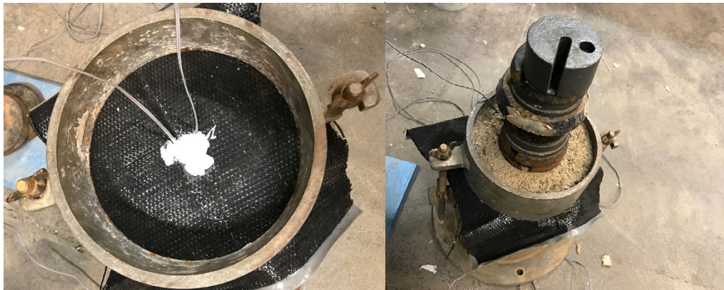
Figure A.4 Initial simplified tests on the effect of boundary condition on the geotextile layer
