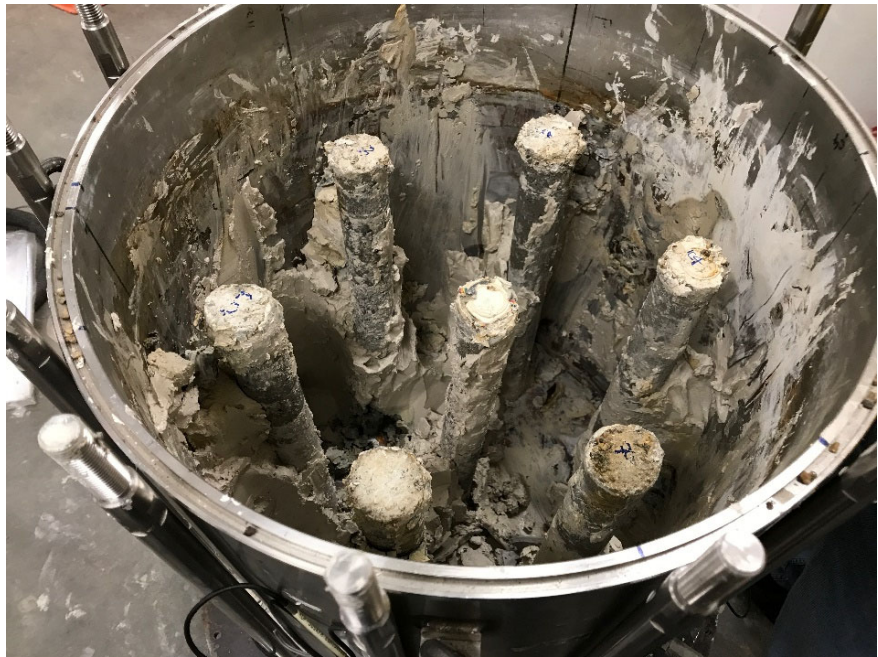
Figure A.8 CICs at the end of the test after the soft soil was excavated
