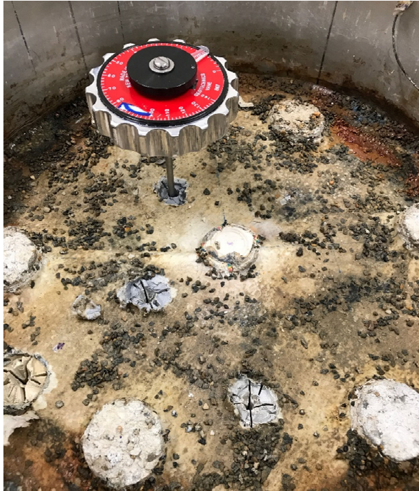
Figure A.9 Vane shear test to determine the shear strength of the soft soil
