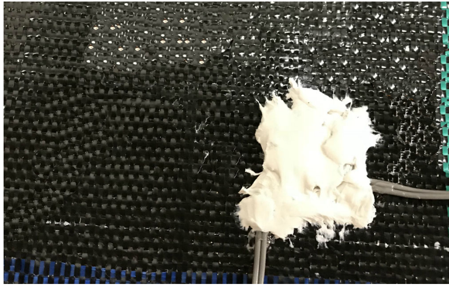
Figure A.5 Butyl rubber (SB) tape applied on the strain gauge to waterproof and protect the gauges
