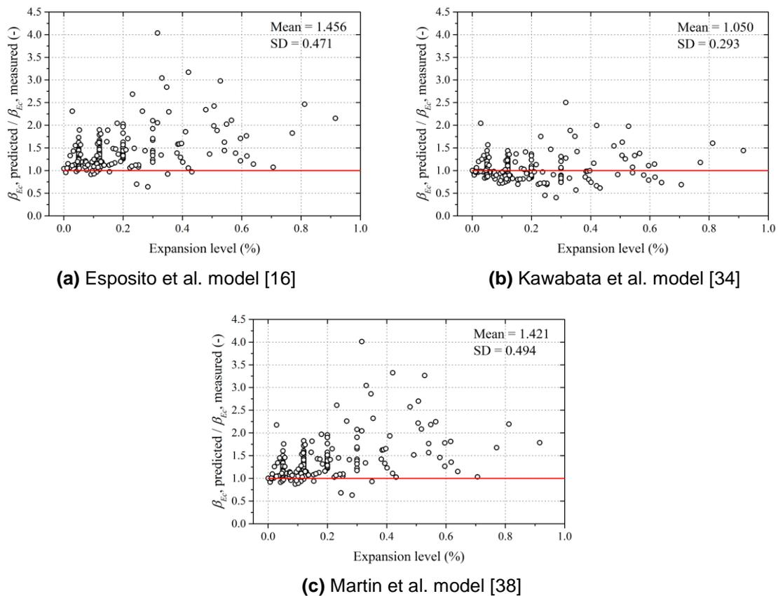
**Figure 4. Comparison of predicted residual elastic modulus from the empirical models to measure data in relation to expansion level**
