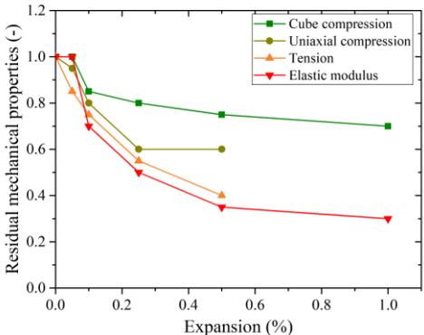
**Figure 1. Lower bound residual mechanical properties as percentage of values for unaffected concrete at 28 days [3]**
