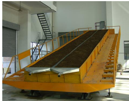
(b) Stationary Soil box with 10 m long, 1.5 m wide and 0.5 m deep
