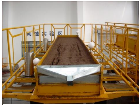
(a) Moveable soil box with 5 m long, 1.0 m wide and 0.5 m deep
