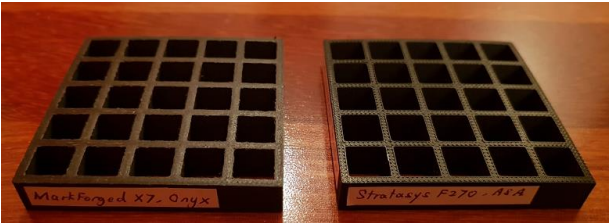
Fig. 1. Print iteration 1: honeycomb structures with thick cell walls made of Onyx (left) and ASA (right). The ASA honeycombs exhibit small defects on the surface.
