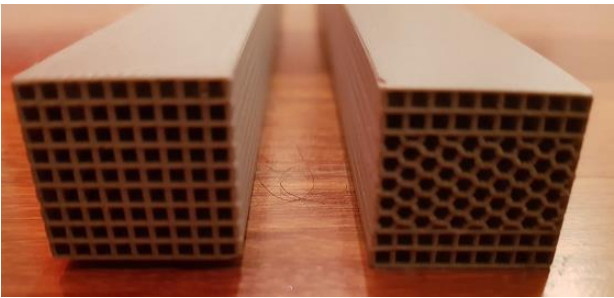
Fig. 2. Cross section profiles of beams with REG and Mix cells using ASA. Note that the cell walls are thinner than those in Figure 1.
