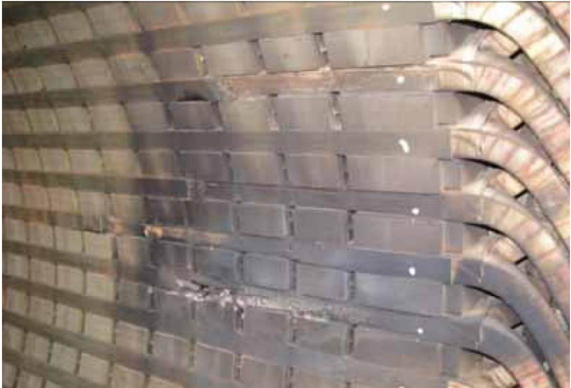
Figure 4-12: Stator winding has an earth fault just below the slot wedge (courtesy of Aurecon).
