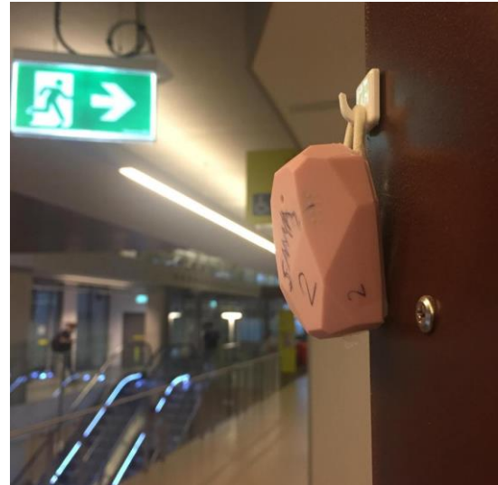
Figure 5.5. Attaching iBeacons on the walls inside the building
