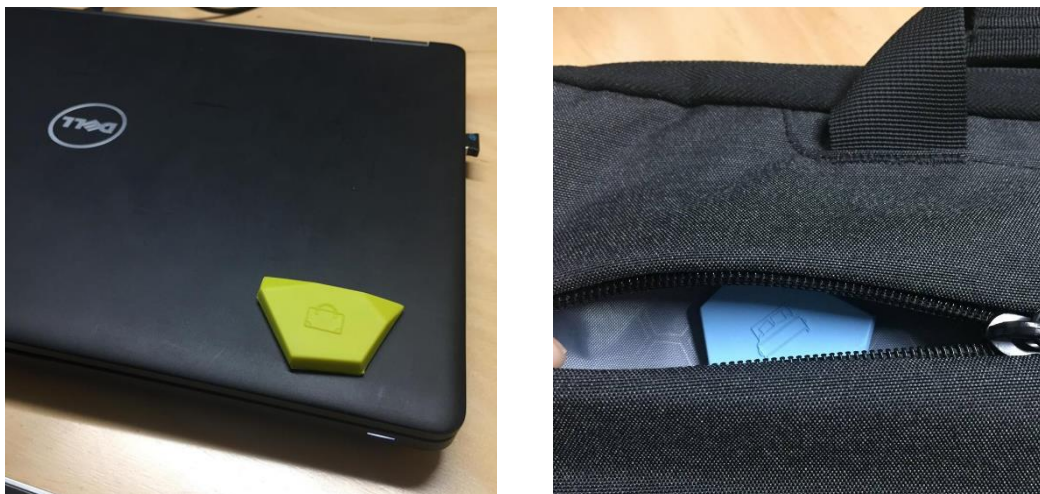
Figure 5.27. Sticking iBeacon on the objects
