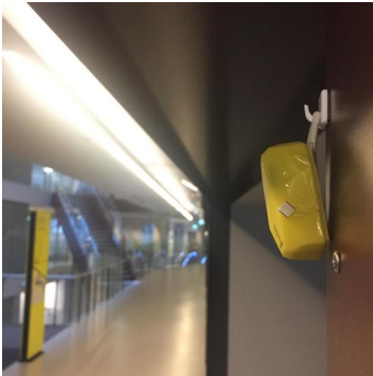
Figure 5.5. Attaching iBeacons on the walls inside the building
