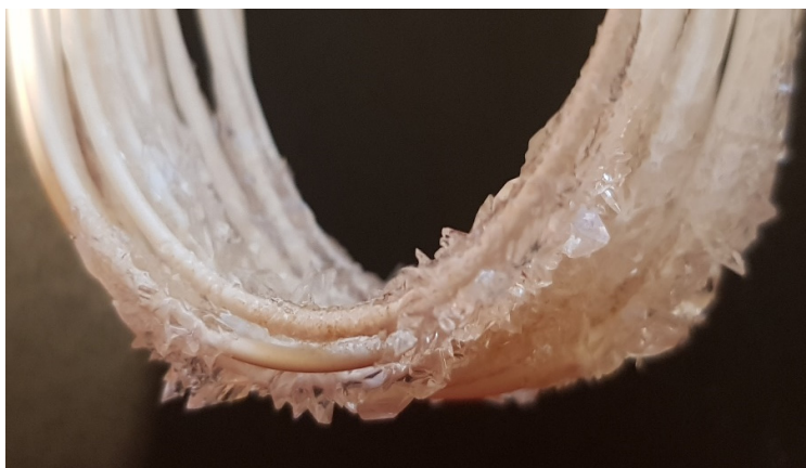
Figure 8-9. Formation of \text{Na}_2\text{SO}_4 crystals on the membrane surface during the period when rapid flux decline was observed.
